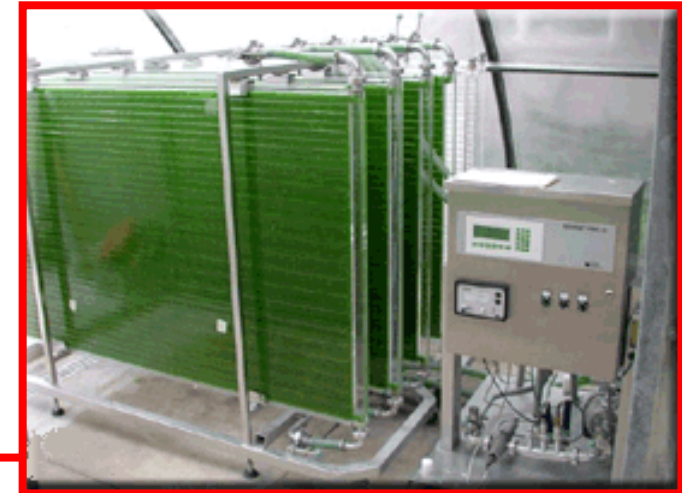
Plan reactor for Chlorella (500 l)
