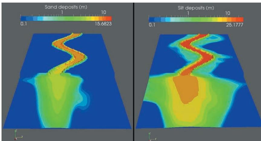
Sand and silt deposits from a multi-event simulation on a synthetic topography with a sinuous channel and downstream unconfined area.
